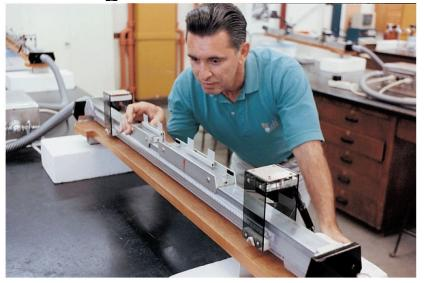
Pucks and carts ride nearly free of friction on cushions of air on air tracks. Galileo worked hard to produce smooth surfaces to minimize friction. How he would have loved to experiment with today's air tracks!
